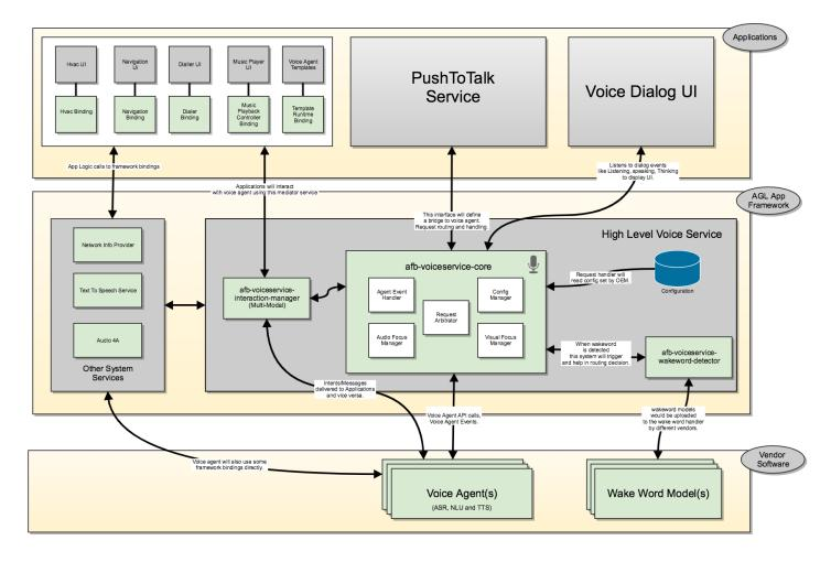
The Voice Services architecture in AGL is layered into two levels. They are High Level Voice Service layer and vendor software layer. In the above architecture, the high-level voice service is composed of multiple bindings APIs (colored in green) that abstract the functioning of all the voice assistants running on the system. The vendor software layer composes of vendor specific voice agent software implementations that complies with the Voice Agent Binding APIs.
